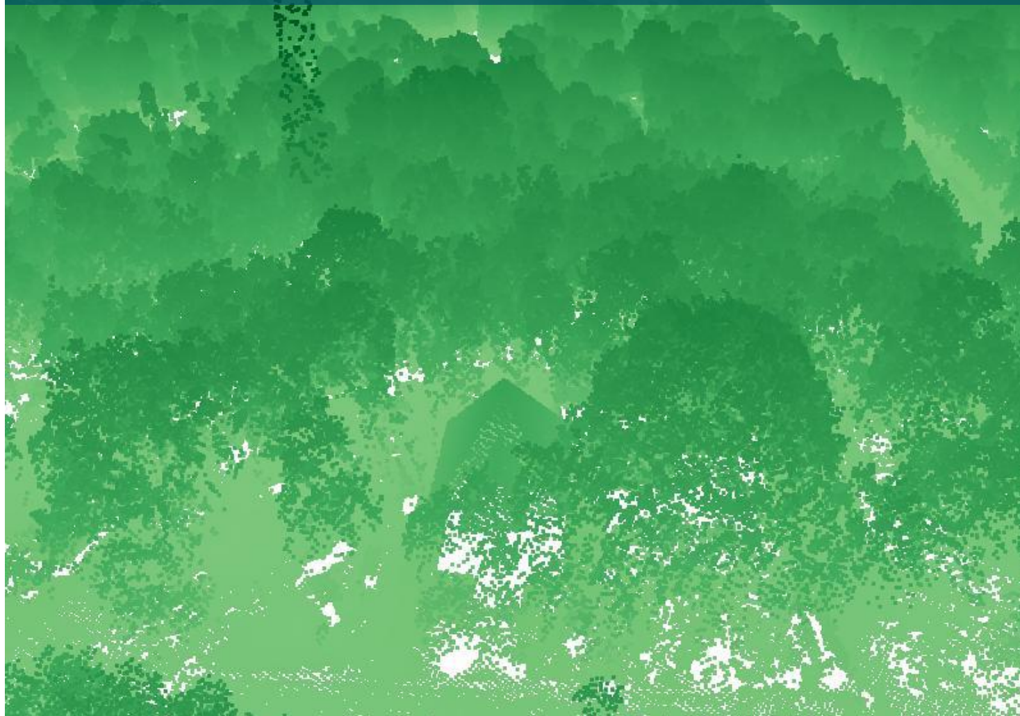
3D LiDAR Elevation Point Cloud
